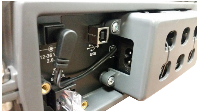
Figure 2.4 AC power block
