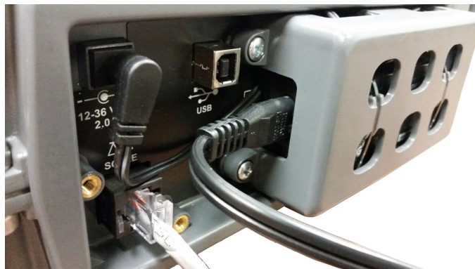
Figure 2.5 AC power connections
